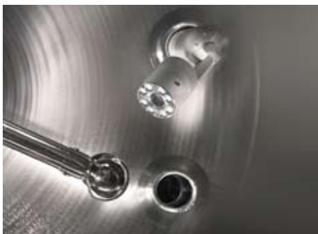
Spray ball coverage inspection for cleaning validation
