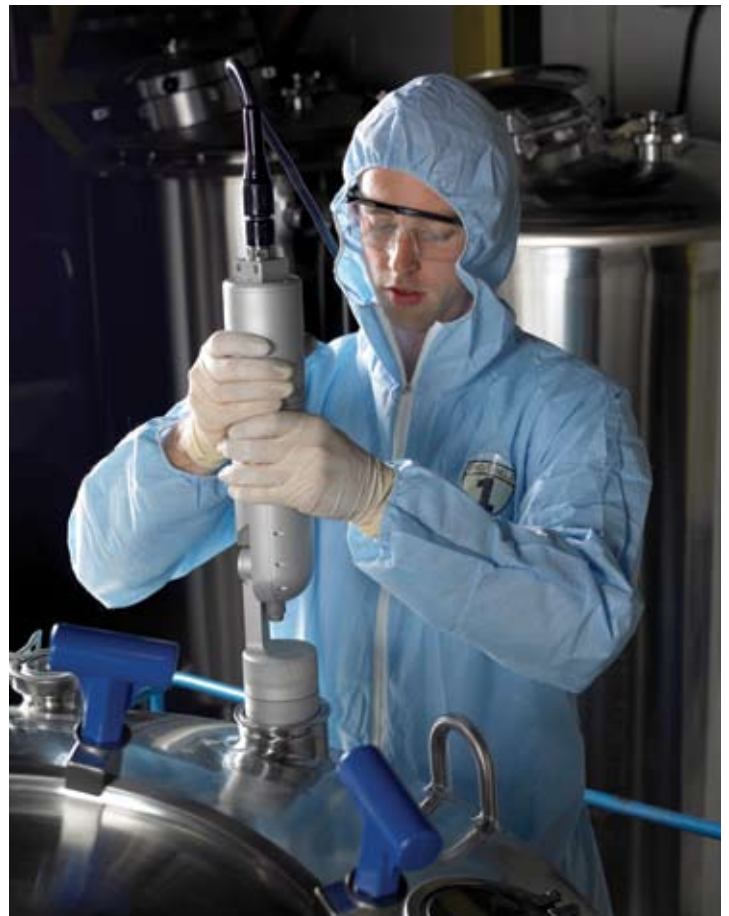
Pharmaceutical tank inspection through 76 mm (3.0 in.) nozzle
